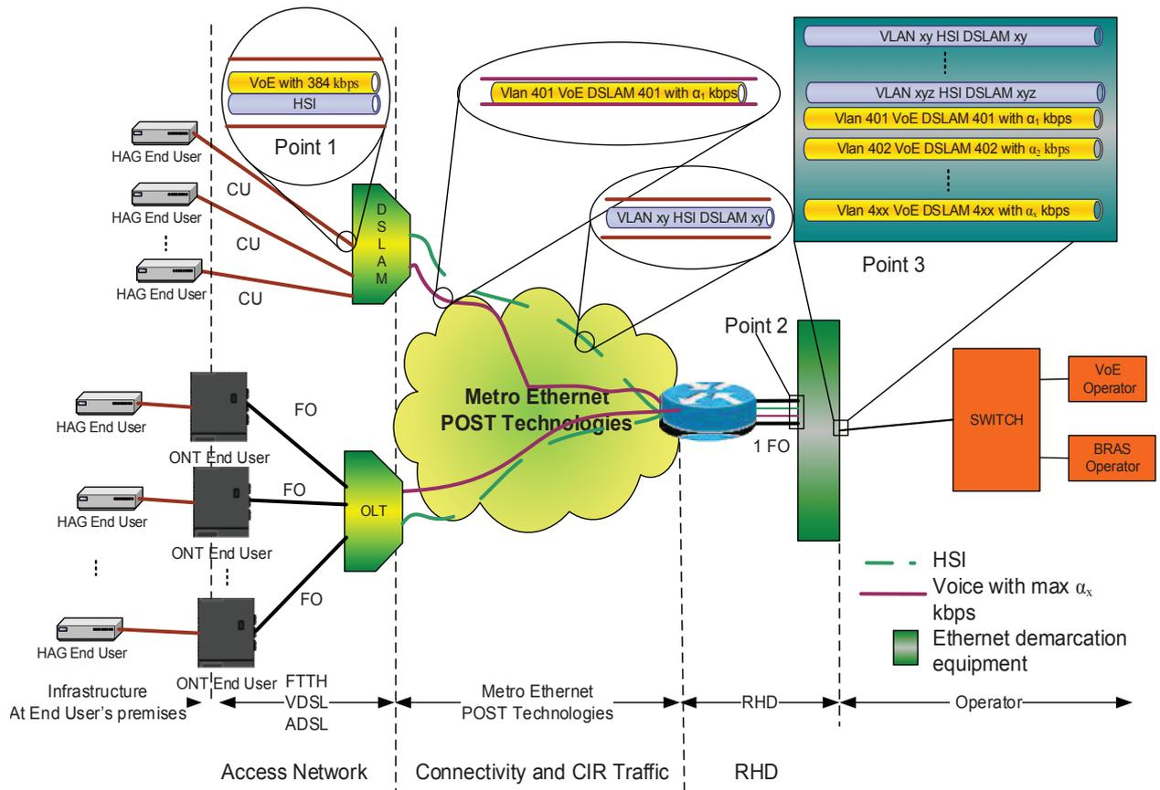
Figure 2: Bitstream Service components in a Multi-VC configuration
