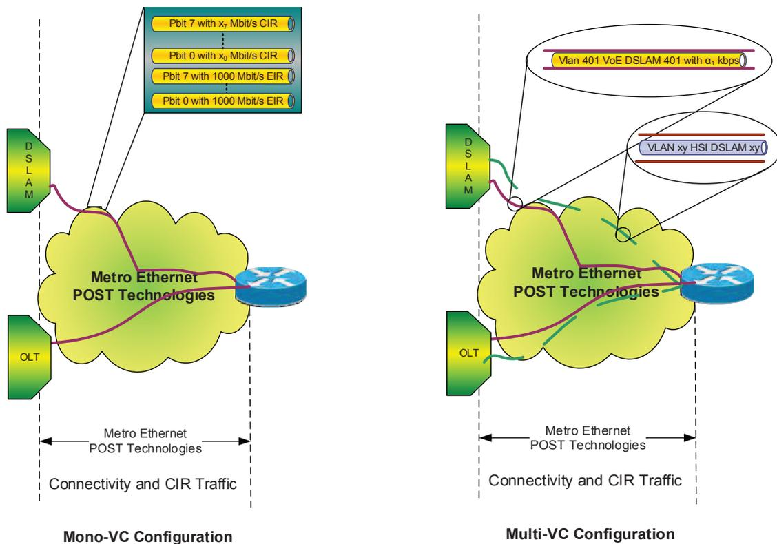
Figure 4: Connectivity component of the Bitstream Service
