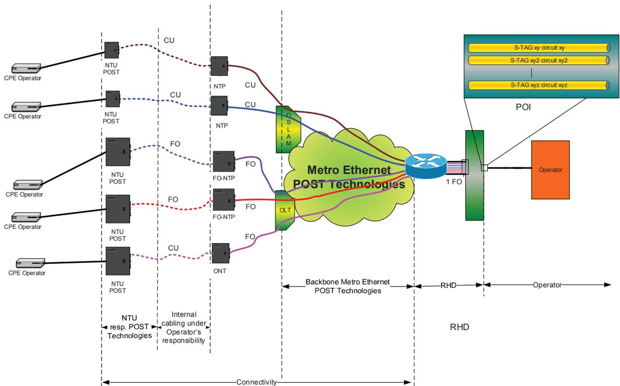
Figure 10: Connectivity component of the EtherConnect Service
