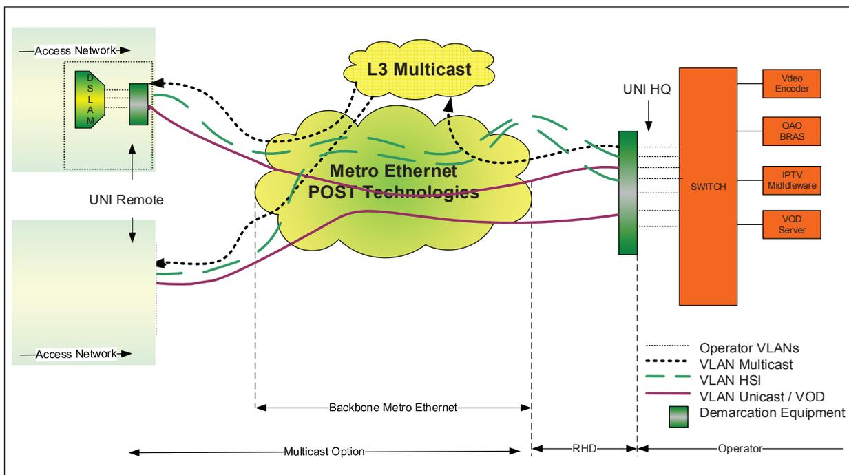
Figure 9: Multicast traffic flow in Multi-VC configurations
