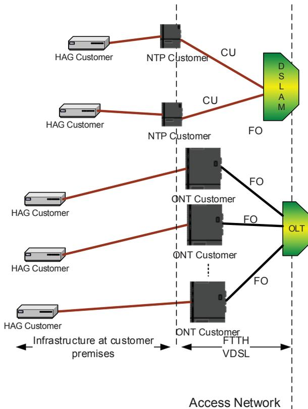
Figure 3: Access component of the Bitstream Service
