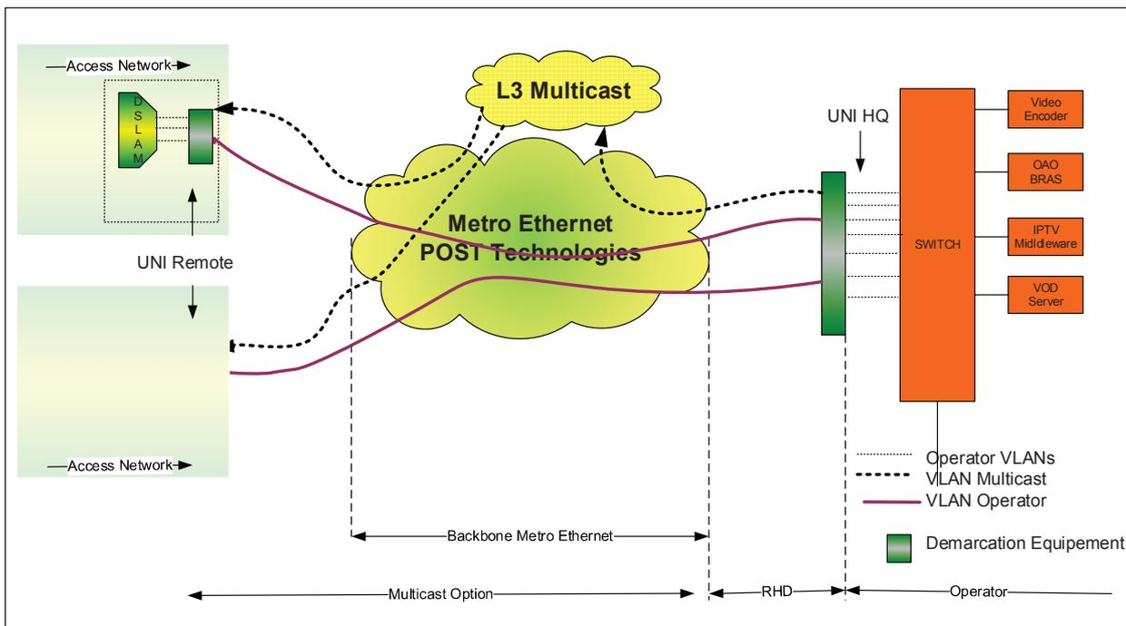
Figure 8: Multicast traffic flow in Mono-VC configurations
