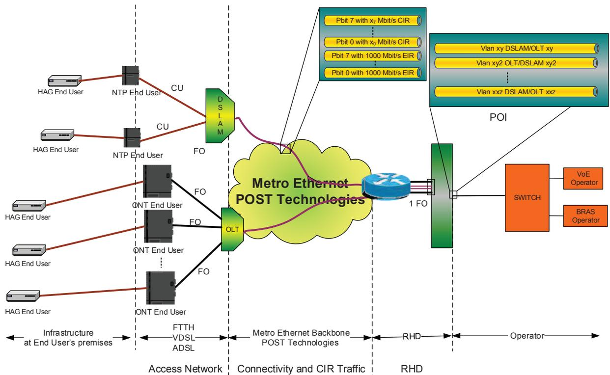
Figure 1: Bitstream Service components in a Mono-VC configuration
