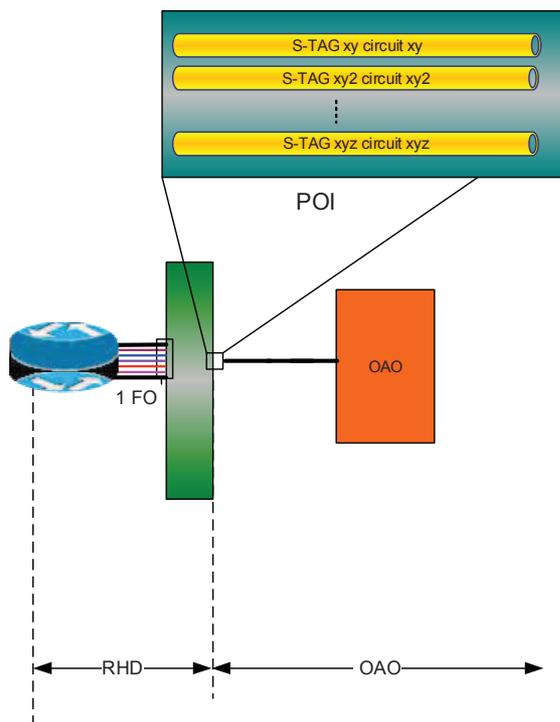
Figure 11: RHD component of the EtherConnect Service
